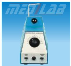
used in the determination of melting of any substance in small quantity upto 300°C. The apparatus is supplied with thermometer and capillaries, operates on 220-240V, 50Hz
