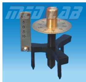
Small, used for measurement of radius of curvature of curved surfaces like lenses etc.
