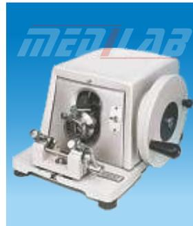
heavy base with knife holder. This Microtome can be set to cut tissue sections from 1 micron to 50 micron thickness. A razor of 120mm is supplied along with. The razor can be tilted upto 30° on a reference scale.
