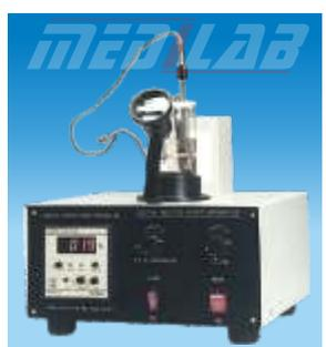
for accurate determination of melting points of solid samples. The unit consists of a built-in magnetic stirrer, an electrode controller for adjusting the rate of heating of silicon oil bath, ON/OFF switch, a pilot lamp, magnifier, a glare free illuminated background, a HIGH/LOW range selector switch and a digital temperature indicator with PT-100 sensor.
