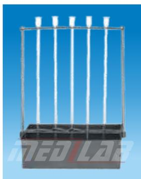
for demonstration of comparison of thermal and volumetric expansion of five different liquids. It has five glass bulbs with funnel shaped mouth, all supported by a metal frame.
