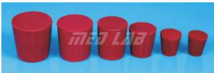
RUBBER STOPPER, with one hole, sizes available from no. 0 to 20
