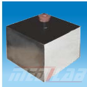
used for qualitative experiments of thermal radiation. This is a sheet metal cube of 13cm with opening at top to fill it with water.
