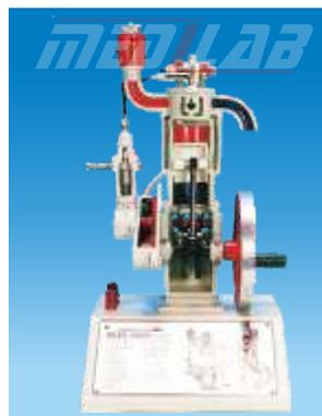
demonstrates functioning of fuel injection system together with hot coil starting device, mounted on a polished wooden base with schematic diagram.
