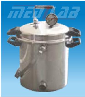
electrical, vertical portable sterilizer, seamless construction using deep drying process, made of heavy duty Stainless Steel, with double safety valve, steam release valve, working pressure 15 lbs, electrical heaters 2kw.
