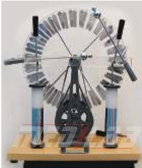
electrostatic generator consists of two 250mm dia discs with radial alluminium segments driven in opposite direction by wheel, with two leyden jars.
