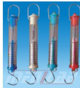
Acrylic, Tubular type, each range is color coded for easy identification, dual scale both in grams and Newton, provision for zero adjustment at top.
