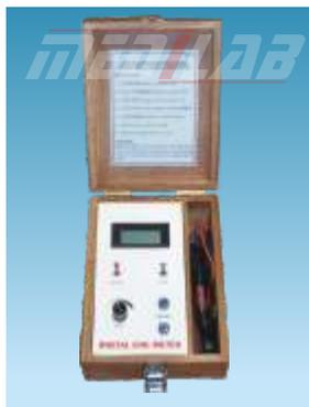
The instrument is for detecting saturation percentage of water in soil. It is workable on 9V battery 3.5 digit display. Complete with 20cm electrode and wooden box.
